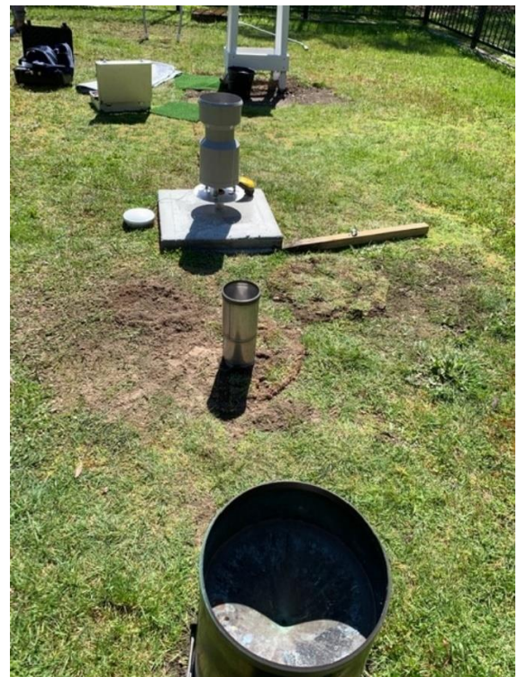
4: Three rain gauges; the two traditional models at the front and the new automatic one at the back
